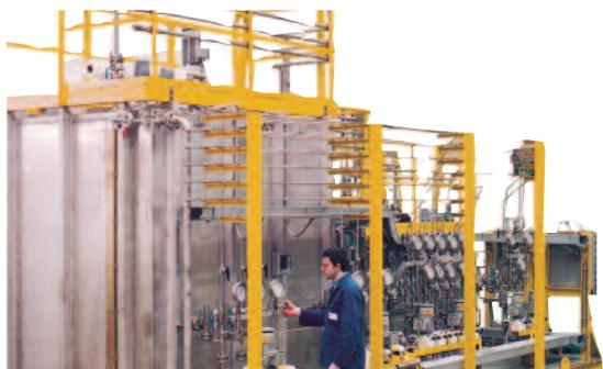
Corrosion inhibitor, Antifoam and Antiscale Injection Package
