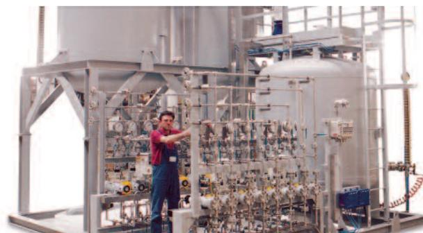
Glycol and Corrosion Inhibitor Injection Package
