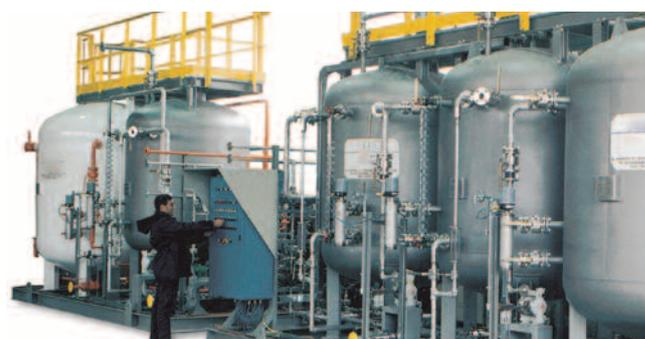
Sulphuric Acid, Biodispersant, Scale Inhibitor and Biocide Dosing Package.
