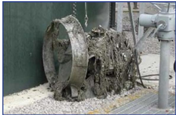
Typical ragged up submersible mixer, which has to be lifted out of the tank for cleaning
